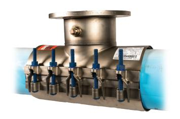
The Triple Tap exceeds industry Standards, AWWA C223 and MSS SP-124-2012. An opposing seal bead system on the upper and lower gaskets combines to provide a secure 360° seal.
