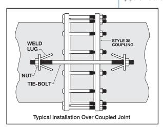
NOTE: Style 440 Joint Harnesses can be custom fabricated for special conditions with larger studs to reduce quantity and installation costs. Use of these products is limited and never required for ordinary conditions. Dresser engineers are glad to assist with project recommendations in all cases of unusual service conditions that may require these devices, and offer the most economical and practical solution for your particular pipe joint requirements.
