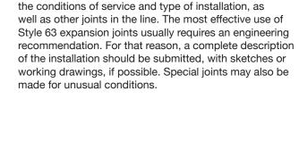
The proper type of expansion joint to use and the method
