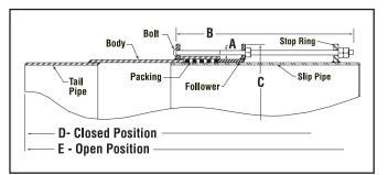
Type 3 is a single-end expansion joint equipped with a limited movement feature to limit the maximum amount of pipe withdrawal. Slip pipes are regularly furnished for Type 3 expansion joints.
