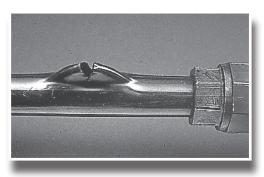
NOTE: Always check insert stiffener to assure it is for wall thickness of tubing being used. (See color code chart at right)
