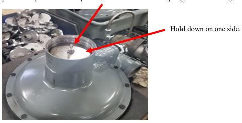
3. Once plate is removed, the main spring will be free to remove and replace with desired spring.
