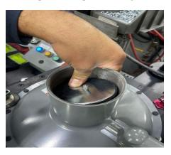
5. Once nut has been started, tighten nut until it stops turning. Nut should be all the way down at this point.
