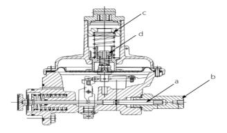
Commissioning SSV1 OPCO - Unscrew the cap (b) and screw it onto the valve rod (a). Slowly pull out the valve rod until the output pressure in the control unit is established, the lever system of the SAV engages and the valve rod remains open. **Only possible if the outlet pressure in the main regulator is less than opco set point!** Then screw the cap (b) back on.
