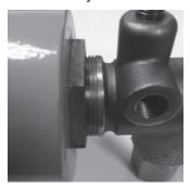
Three to five threads of the fluid head assembly should be visible once it has been installed onto the main pump body.
