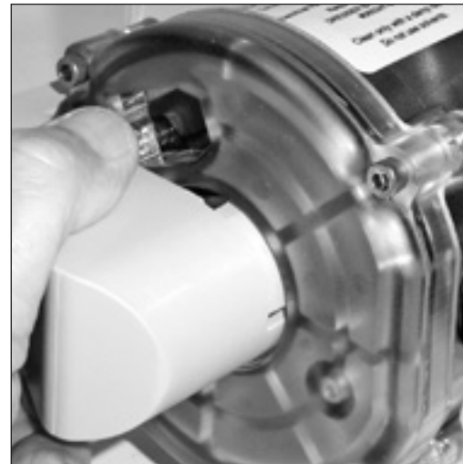
Figure 10.35 - Place cable gland connector into recess
