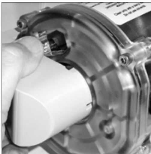
Figure 10.38 - Place cable gland connector into recess
