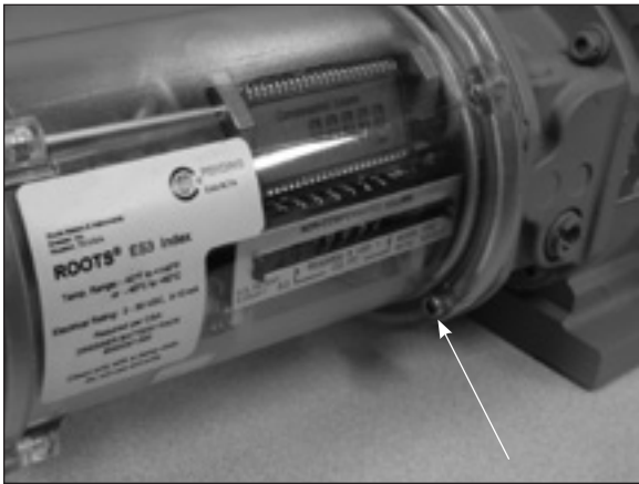
Figure 10.27 - Insert the 3/4-inch (short) screw
