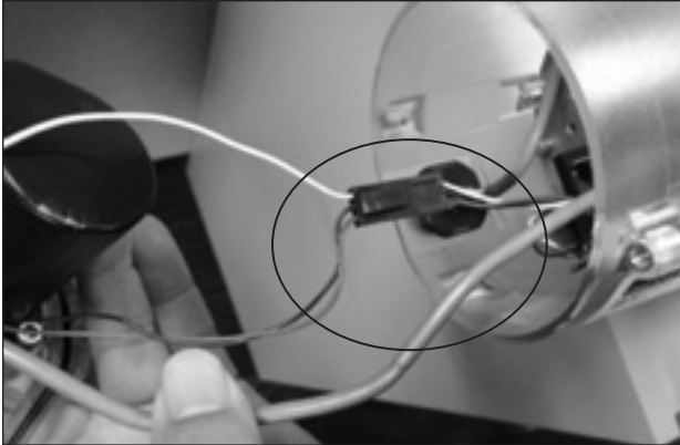
Figure 13.1 -Squeeze to release cord
