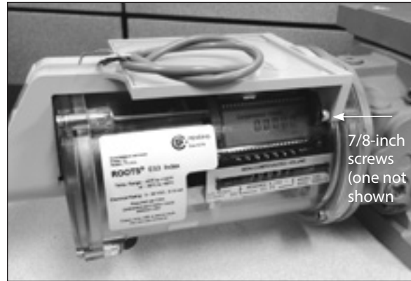
Figure 10.29 - Insert the 7/8-inch (long) screws
