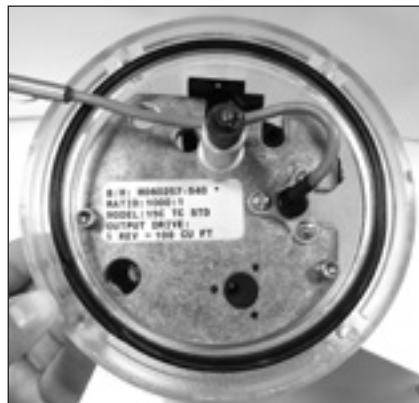
Figure 10.19 - Quad-Ring seal in circular groove
