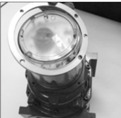
Figure 10.2 - Remove slip flange
