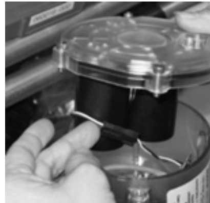
Figure 13.3 -Remove excess slack: circular version
