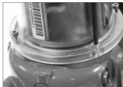
Figure 10.12 - Torque mounting screws to a maximum of 12-14 inch-pounds
