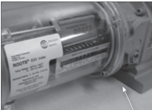
Figure 10.23 - Insert the 3/4 inch (short) screw
