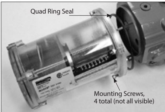
Figure 10.8 - Exploded view of assembling the ES3 on Series B meters
