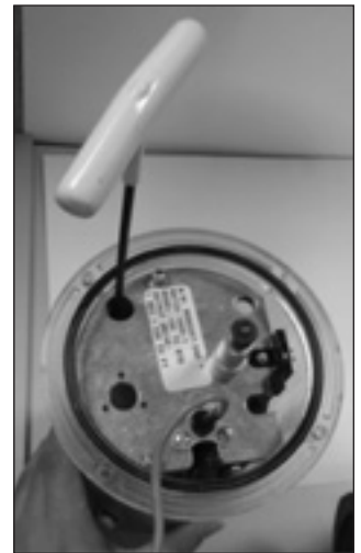
Figure 13.10 - Remove single screw holding counter to unit
