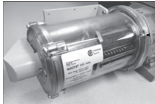
Figure 10.26 - Insert remaining 3/4 inch (short) screws
