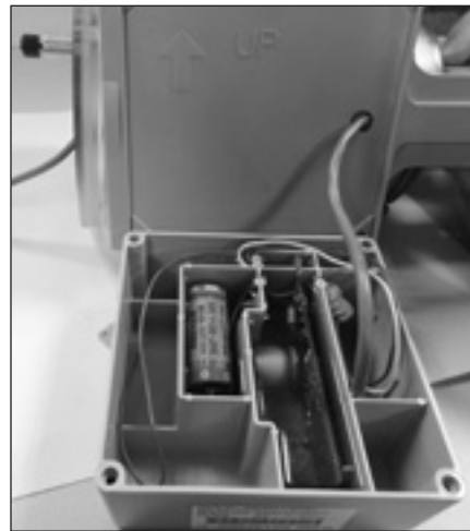
Figure 11.14 - Tuck extra cable into a pocket
