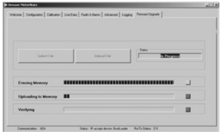
Figure 15.8 - Progression of three steps for uploading the new firmware to the unit
