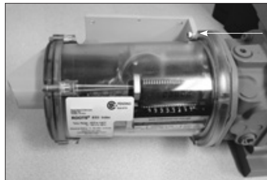
Figure 10.36 - Insert the 7/8-inch (long) screws
