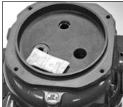
Figure 10.4 - New desiccant pack in place
