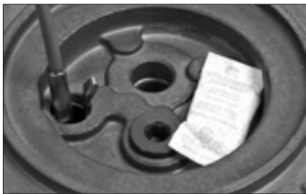
Figure 10.20 - Insert Temperature probe
