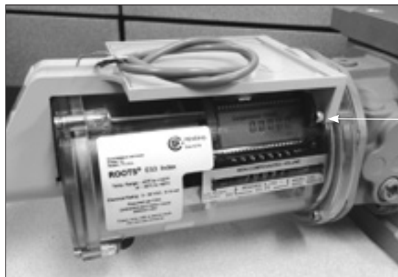
Figure 10.39 - Insert the 7/8-inch (long) screws
