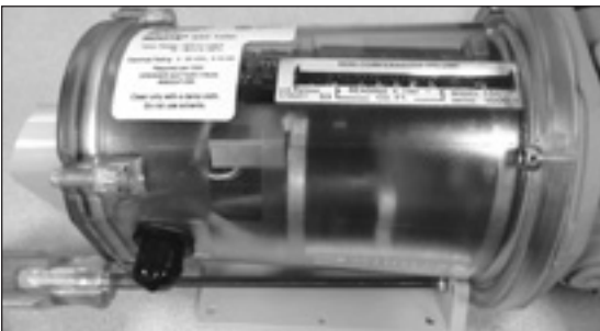
Figure 10.33 - Remove screws attached to AMR bracket
