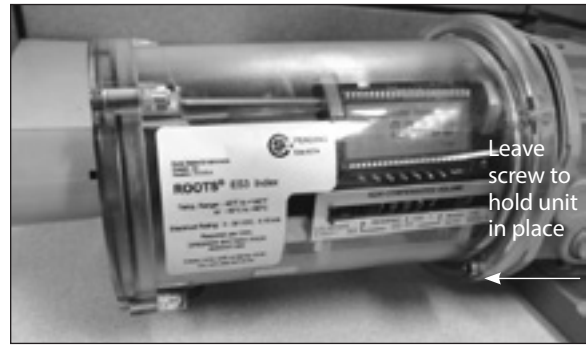
Figure 10.34 - Leave screw under odometer in place
