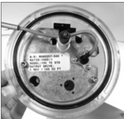
Figure 10.9 - Quad-Ring seal in circular groove
