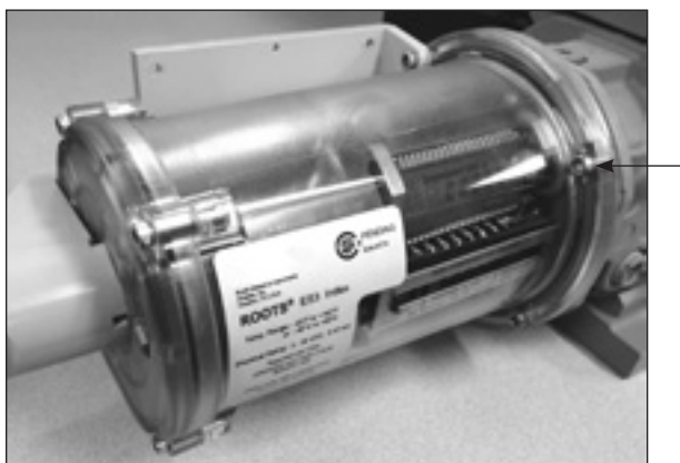
Figure 10.37 - Insert the 3/4-inch (short) screw
