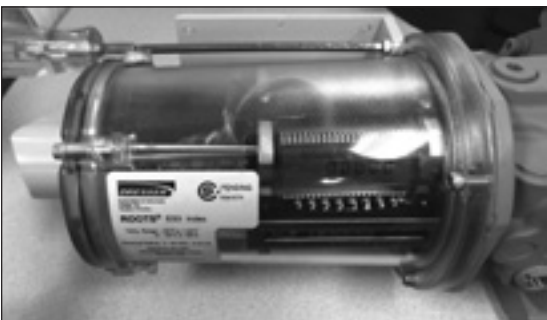
Figure 10.32 -Remove screws attached to AMR bracket
