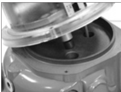
Figure 10.21 - Seat magnet in magnet well
