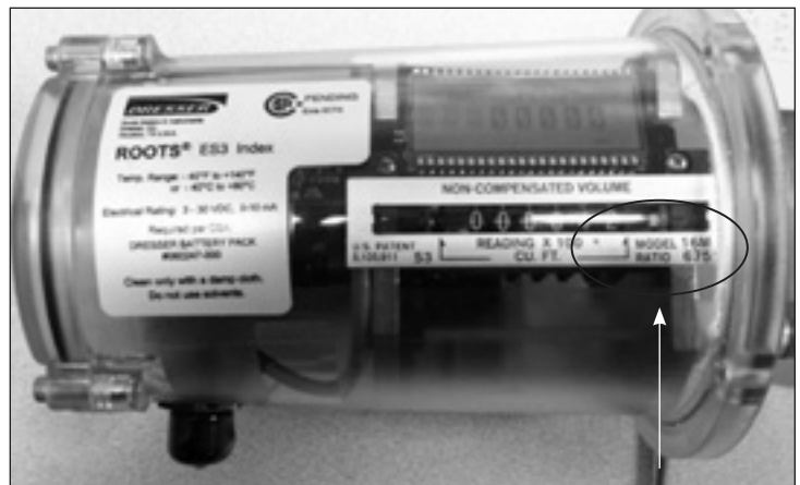
Figure 12.1 - Location of meter size and gear ratio Meter size = 16M Ratio = 675
