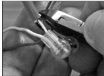
Figure 11.13 - Clip unused wires
