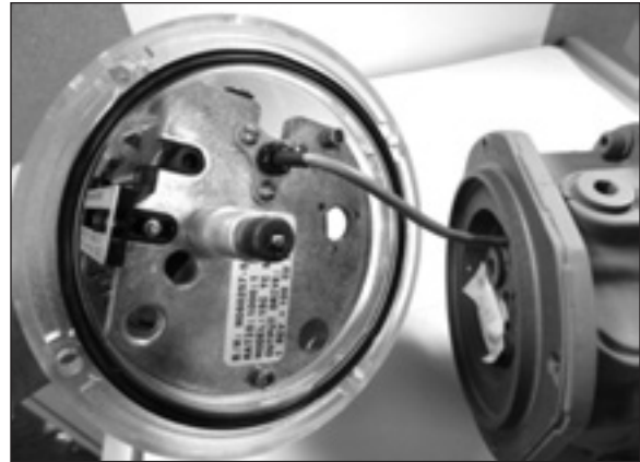
Figure 13.9 - Remove grommet securing previous probe; remove plate for probe
