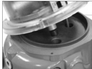
Figure 10.11 - Seat magnet in magnet well
