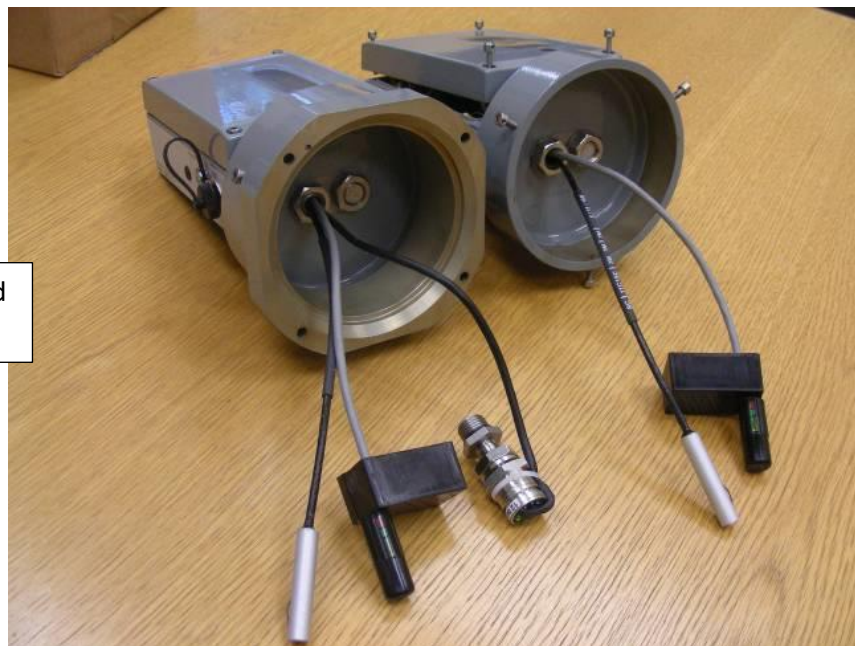
Temperature Probe and Pressure Transducer
