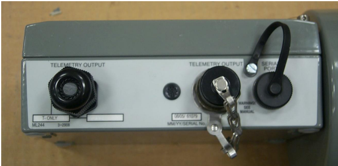
Example of a Cable Gland and Military Style Circular Connector
