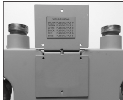
Figure 7.10 -Properly positioned mounting bracket
