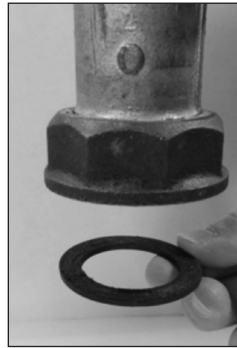
Figure 5.1 - Proper installation of washer into swivel
