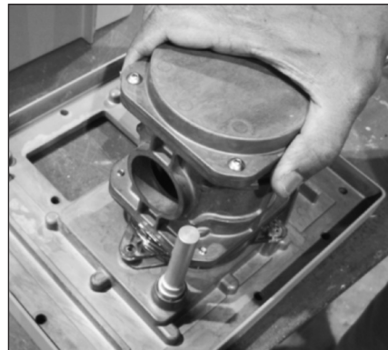
Figure 16.10 Example - Proper alignment of measurement cartridge
