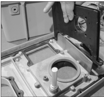
Figure 16.8 Example - Remove main gasket
