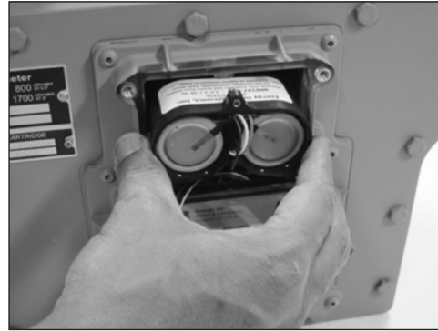
Figure 9.21 Example - Place battery inside compartment
