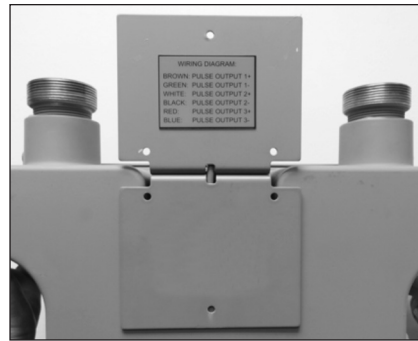
Figure 7.17 Example - Properly positioned mounting bracket
