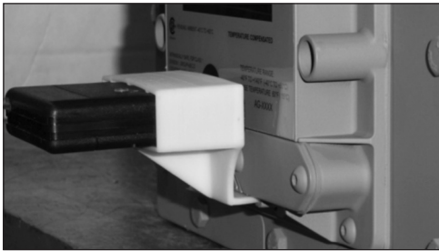
Figure 10.15 Example - IrDA adapter placed into slot
