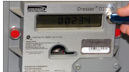
Figure 6.2 Example - Swipe magnet across the black dot to change the screens
