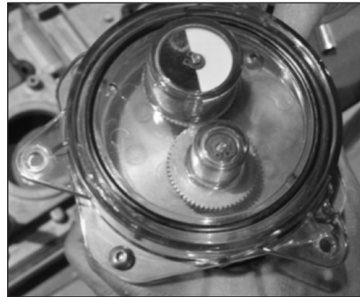
Figure 16.9 Example - Place O-ring on amber cartridge cover
