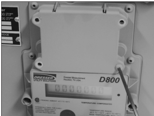
Figure 9.7 Example - Remove 4 screws on battery compartment
