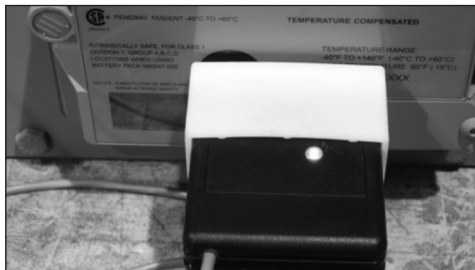
Figure 10.17 Example - Light indicating connection established
