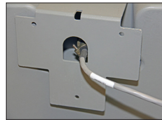
Figure 7.18 Example - Pull cable through the center hole
