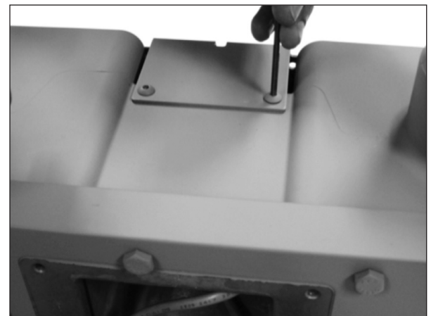
Figure 9.10 Example - Remove AMR plate
