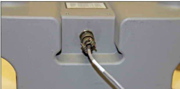
Figure 7.16 Example - Pulse output with male mating pigtail connection installed
