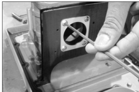
Figure 16.6 Example - Remove 4 (#10-24) screws on main gasket
