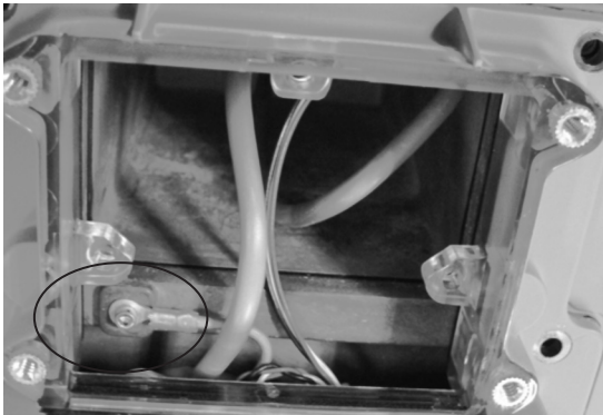
Figure 9.18 Example - Attach green ground wire
