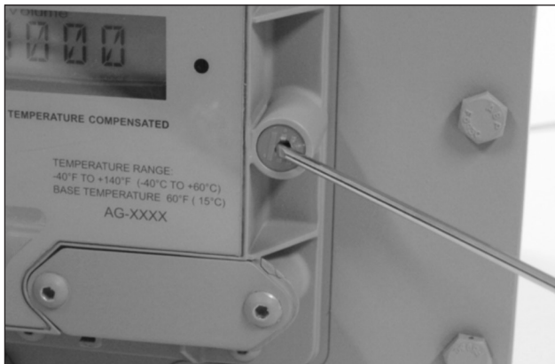
Figure 9.6 Example - Remove rock seals.
