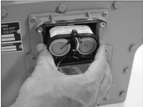
Figure 9.28 Example - Remove battery pack
