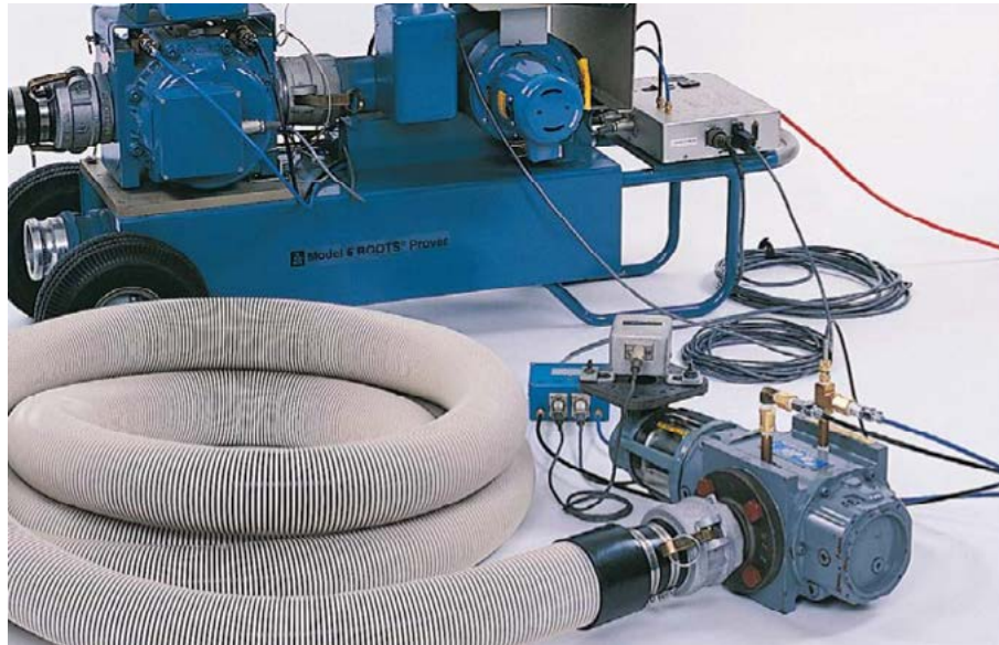
Figure 5: Instrument Drive Pulser test set-up.
