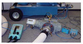
Meter and corrector combined accuracy measurement system including; Model 5 Prover, SmartProve™ Interface and external reference pressure source.
