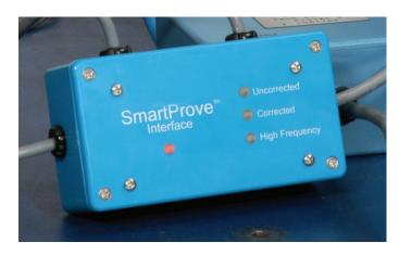
The Dresser Utility Solutions Model 5 Transfer Prover, equipped with the SmartProve™ Interface Cable, is a fully integrated, computer controlled system that can test the combined accuracy of the Dresser rotary gas meter and the Dresser Micro Corrector; model IMC/W2 integral mount and model MC2 instrument drive mount.
