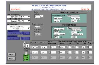
The prover operator only has to press the START button to initiate the test, which is then automatically performed at all the pre-selected test flow rates.
