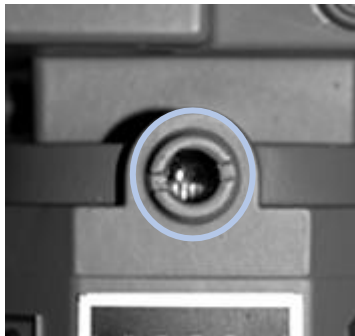
Figure 3: Flow Indicator location under cover in meter
