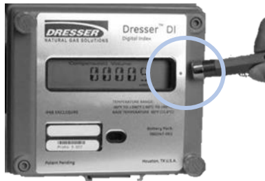
Figure 2: Magnet used to change screens
