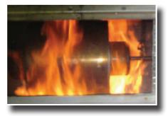
Dresser couplings were subjected to a 30 minute fire test at 1472°F (800°C), in accordance with ABS Rules and meet ISO 19921 and ISO 19922 requirements.
