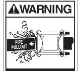
When pipe pullout could occur, pipe joint MUST be anchored. Failure to anchor pipe joint could result in escaping line content and cause property damage, serious injury or death.
