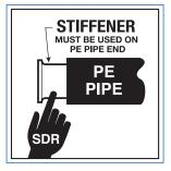
NOTE: On all polyethylene pipe ends, the recommended Dresser insert stiffener, or an insert stiffener the user has qualified to meet CFR Title 49, DOT 192.283(b), must be installed.
