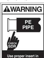
Use proper insert in PE pipe end.
