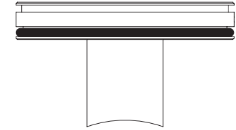
Scarfed nipple completion plug* available for replacing coupon in tapped hole
