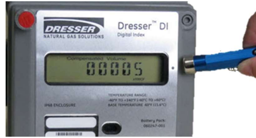
Figure 17: Series D/Series K: Swipe magnet vertically across the black dot by the LCD screen
