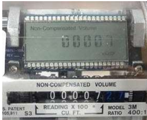
Figure 22: Non-compensated index matching LCD screen
