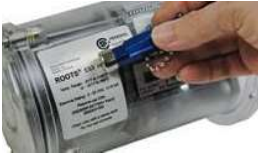
Figure 16: ES3/ETC Index: Swipe magnet along the Swipe line
