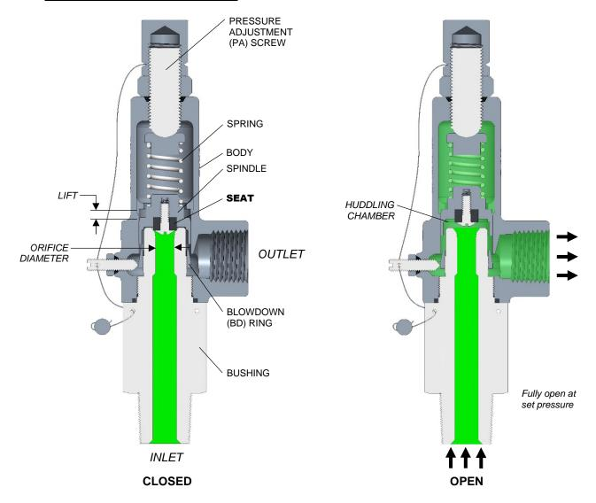
The FLOW SAFE F80M Series safety relief valve is a direct-acting spring-loaded relief valve, suitable for gas service. The Type F84M is plastic-seated and the F85M is elastomer-seated.
