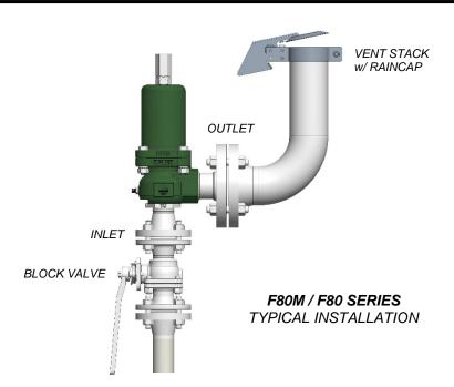
The F80M Series valves are **not** balanced against superimposed backpressure, so that the set pressure will change one-for-one with the backpressure. This means that for each 1 psi of backpressure, the set pressure will increase by 1 psi. Refer to Section 4.3 for setting instructions. **Check the valve manufacturer's nameplate(s) to determine if the valve was already set with a correction for backpressure**.
