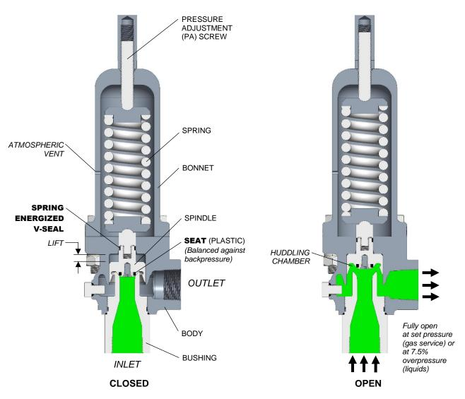
The FLOW SAFE F88 Series safety relief valve is a direct-acting spring-loaded relief valve, suitable for gas and/or liquid service. The Type F88 is plastic-seated with a plastic seal.
