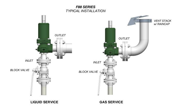
Ensure that the inlet piping/flanges have an opening equal to or greater than the valve's inlet diameter. Make sure that there are no obstructions such as gaskets, fittings, etc., in the flow path to restrict the flow or cause chatter. Also, misaligned piping connections may result in leaks or induce stresses in the valve assembly that interfere with good operation. Discharge stacks exposed to the elements should be configured so as to avoid the accumulation of ice and snow.
