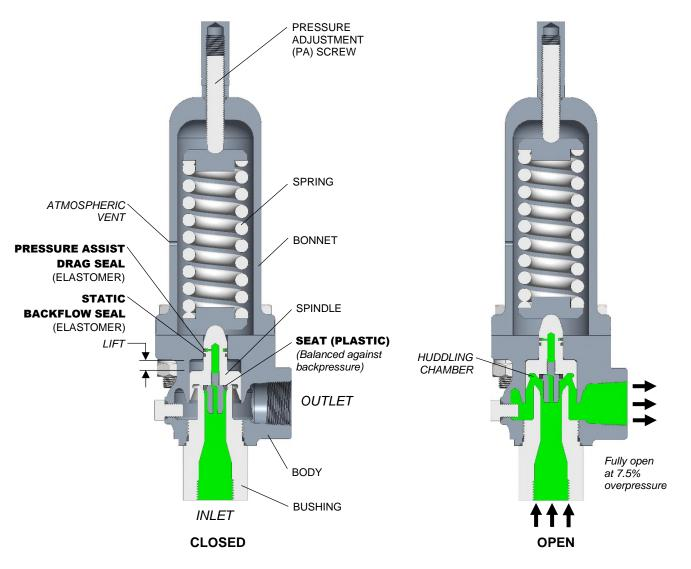
The FLOW SAFE F84L Series liquid relief valve is a direct-acting spring-loaded relief valve, suitable for liquid service. The Type F84L is plastic-seated with elastomeric seals.
