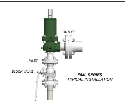
The F84L Series valves are balanced against superimposed backpressure, so that the set pressure will not change with backpressure.
