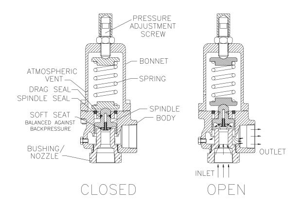
The FLOW SAFE F84L Series liquid relief valve is a direct-acting spring-loaded relief valve, suitable for liquid service. The Type F84L is plastic-seated with elastomeric seals.
