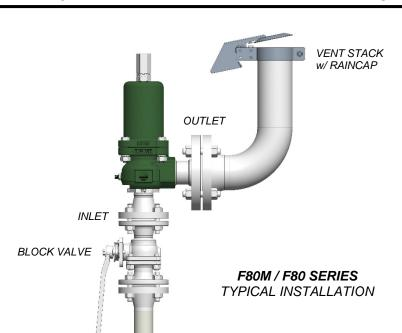
The F80M Series valves are **not** balanced against superimposed backpressure, so that the set pressure will change one-for-one with the backpressure. This means that for each 1 psi of backpressure, the set pressure will increase by 1 psi. Refer to Section 4.3 for setting instructions. **Check the valve manufacturer's nameplate(s) to determine if the valve was already set with a correction for backpressure**.
