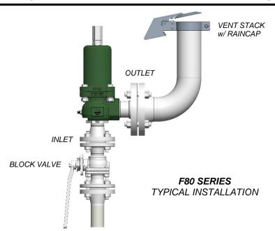
The F80 Series valves are **not** balanced against superimposed backpressure, so that the set pressure will change one-for-one with the backpressure. This means that for each 1 psi of backpressure, the set pressure will increase by 1 psi. Refer to Section 4.3 for setting instructions. **Check the valve manufacturer's nameplate(s) to determine if the valve was already set with a correction for backpressure**.
