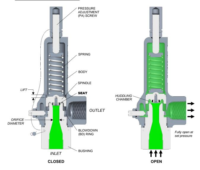
The FLOW SAFE F80 Series safety relief valve is a direct-acting spring-loaded relief valve, suitable for gas service. The Type F84 is plastic-seated and the F85 is elastomer-seated.
