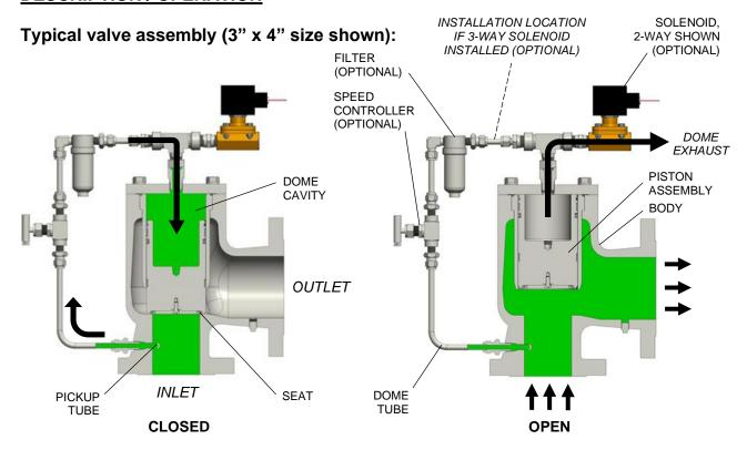
The FLOW SAFE F70U Series unloader valve provides a means to control flow for a variety of process flow applications, such as compressor and blower unloading. It is designed to be repeatedly cycled at full pressure throughout its range of rated temperatures.
