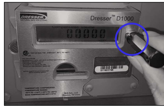
Figure 2: Swipe magnet across black dot to change the screen
