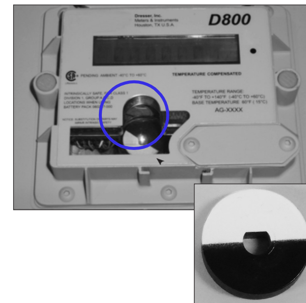
Figure 3: RPM Wheel location under cover in meter
