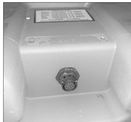
Figure 22: Pulse output cable connection on backside of meter
