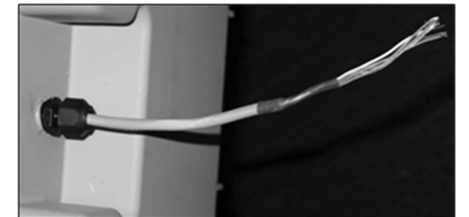
Figure 19: Loosen cable gland and extend the cable out of the gland
