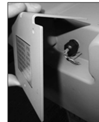
Figure 34: Pulse output cable under the protective plate
