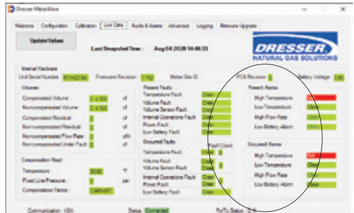
Figure 10.3 -Live Data Screen showing Alarms in Dresser MeterWare Software
