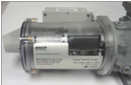
Figure 9.17 -Top inlet: notice the space between the ETC label and the bracket
