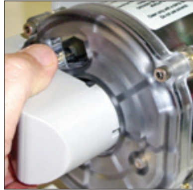
Figure 8.58-Place cable gland connector into recess
