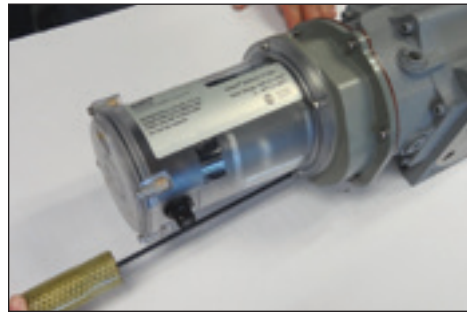
Figure 8.24 -Torque mounting screws to a maximum of 12-14 inch-pounds
