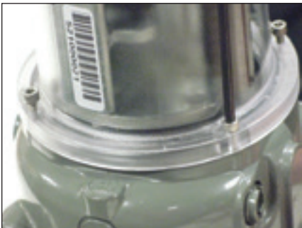
Figure 8.12 -Torque mounting screws to a maximum of 12-14 inch-pounds.
