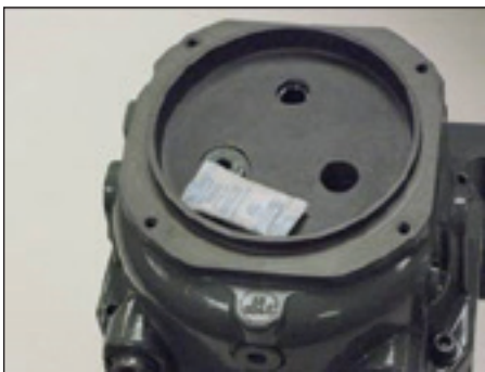
Figure 8.6-New desiccant pack in place
