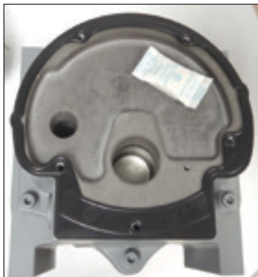
Figure 8.18 -Interface gasket placed on meter body
