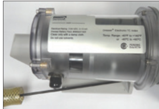
Figure 8.53-Remove screws attached to AMR bracket
