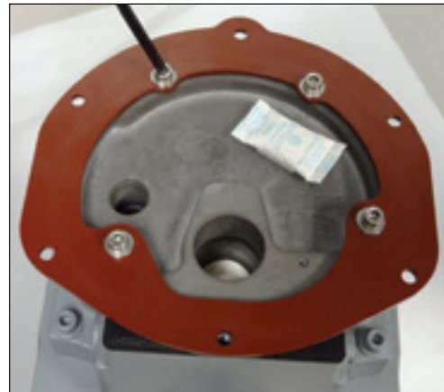
Figure 8.37 -Adapter Plate installed on meter body.
