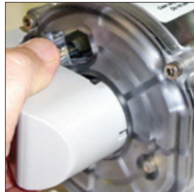
Figure 8.48 -Place cable gland connector into recess
