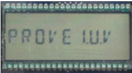
Figure 12.10-LCD screen changes to PROVE I.U.V
