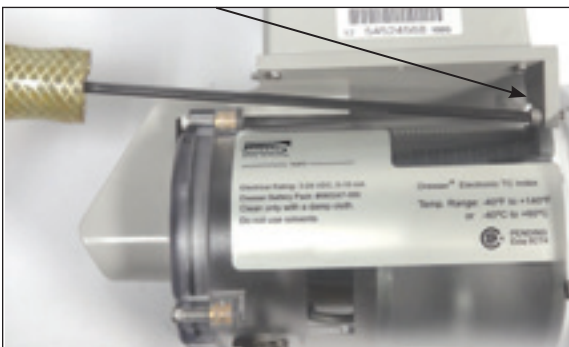
Figure 11.4- Remove two screws attaching AMR bracket to ETC
