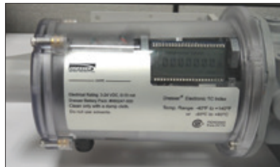
Figure 8.54-Leave screw under odometer in place
