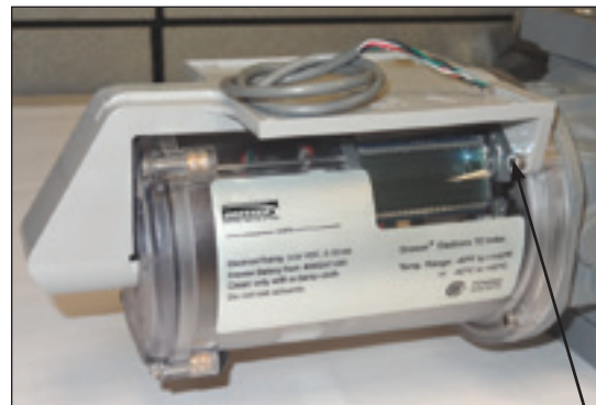
Figure 8.49 -Insert the 7/8-inch (long) screws 7/8" screws (one not shown)
