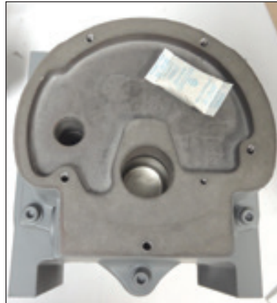
Figure 8.13 -New desiccant pack in place.
