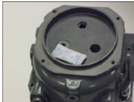
Figure 8.25 -New desiccant pack in place
