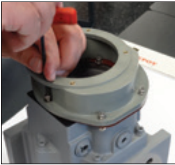
Figure 8.22 -Install cap screws, washers and hex lock nuts.
