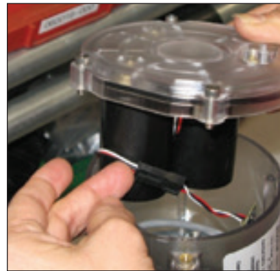
Figure 11.3-Remove excess slack: circular version
