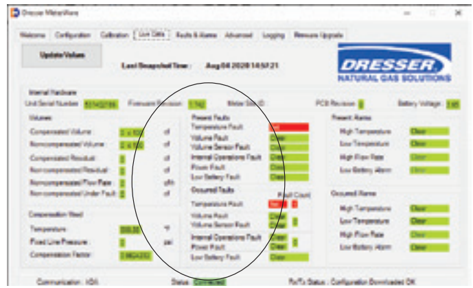
Figure 10.2 -Live Data Screen showing Faults in Dresser MeterWare Software
