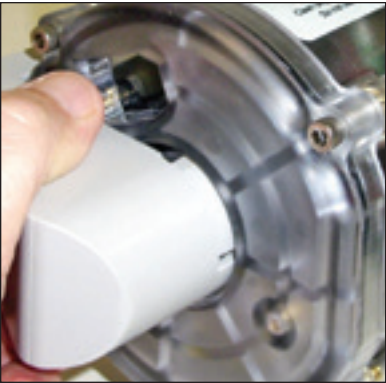
Figure 8.55-Place cable gland connector into recess
