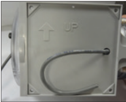
Figure 9.9-Cut the AMR cable
