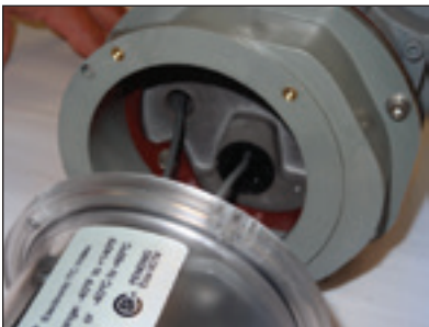
Figure 8.23 -Seat mag pick-up in magnet well
