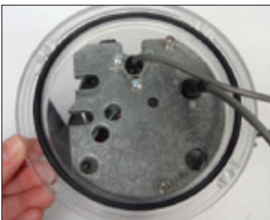
Figure 8.35 -Orange O-ring seal seated in circular groove
