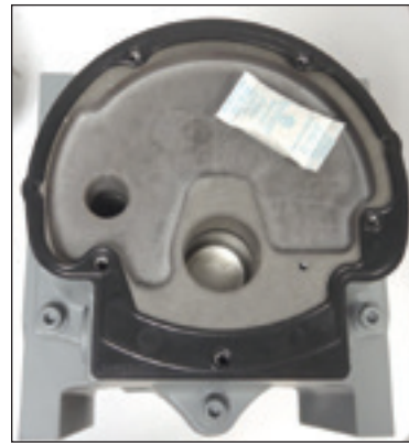
Figure 8.36 -Interface gasket placed on meter body
