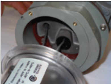
Figure 8.41 -Seat mag pick-up in magnet well
