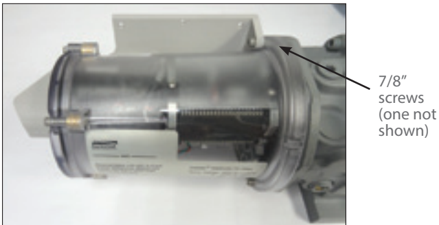
Figure 8.45 -Insert the 7/8" (long) screws
