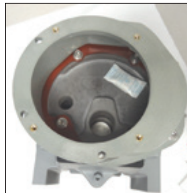
Figure 8.21 -Lexan Adapter Housing placed on top of the adapter plate.
