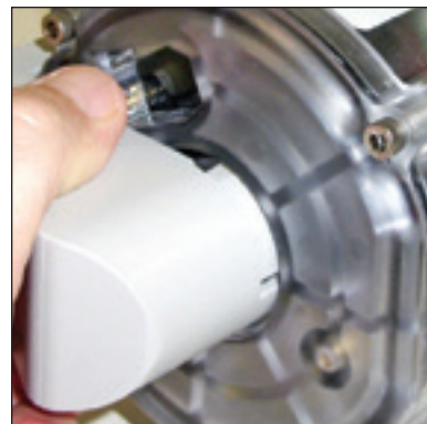
Figure 8.44 -Place cable gland connector into recess
