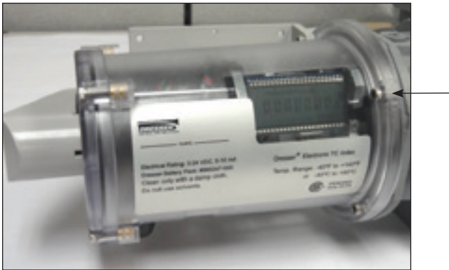
Figure 8.46 -Insert the remaining 3/4 inch (short) screw
