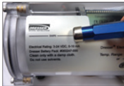
Figure 7.2-Swipe magnet across the swipe line to change the screen displays
