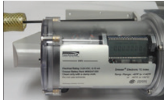
Figure 8.52-Remove screws attached to AMR bracket
