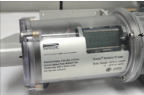
Figure 8.57-Insert the 3/4-inch (short) screw
