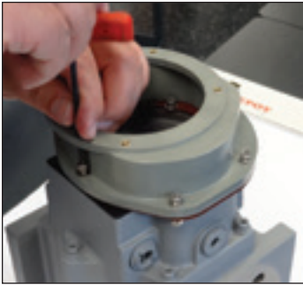
Figure 8.40 -Install cap screws, washers and hex lock nuts.
