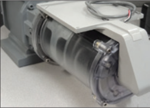
Figure 8.60-Insert the 3/4-inch (short) screw
