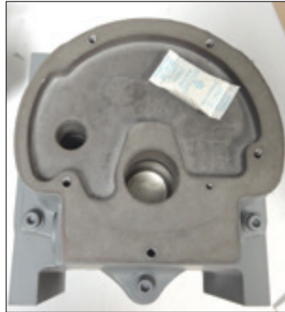
Figure 8.31-New desiccant pack in place.
