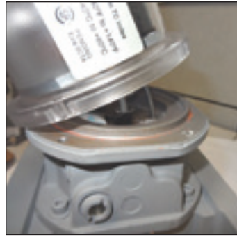
Figure 8.30-Seat mag pick-up in magnet well
