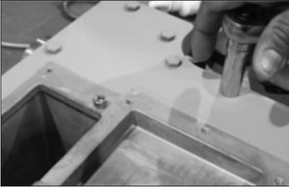
Figure 9.32 - Retirez les 16 boulons
