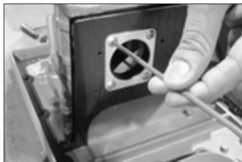
Figure 9.37 - Retirez 4 vis (#10-24) du joint principal
