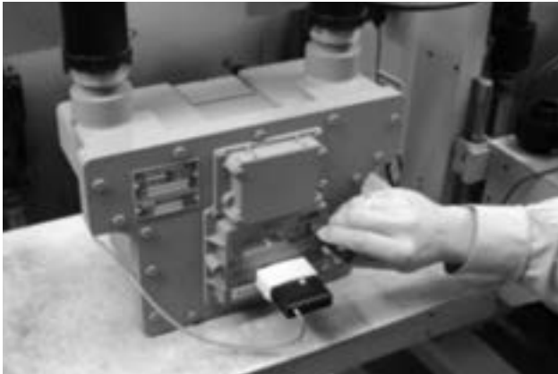
Figure 10.13 Example - Light on IrDA cable indicates connection is established
