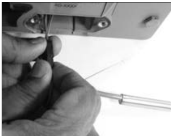
Figure 9.3 Example - Press and release the black connector to remove temperature probe
