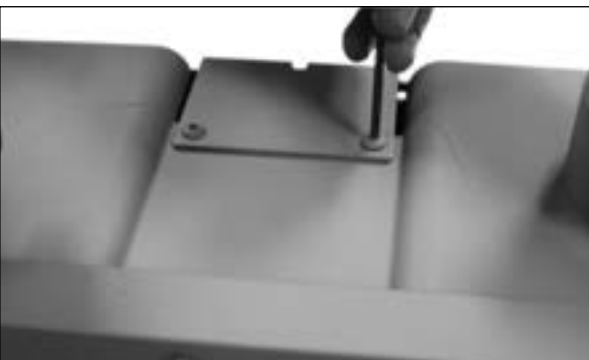
Figure 9.25 Example - Attach AMR plate to the meter.
