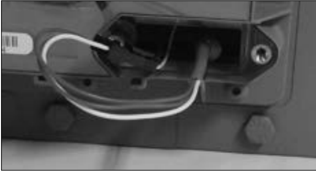
Figure 9.23 Example - Push temperature probe into probe well
