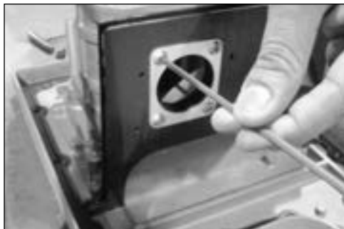
Figure 16.6 Example - Remove 4 (#10-24) screws on main gasket
