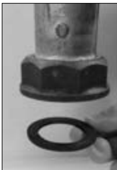
Figure 7.1 Example - Proper installation of washer into swivel
