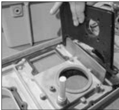
Figure 16.8 Example - Remove main gasket
