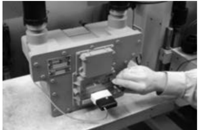
Figure 10.14 Example - Light on IrDA cable indicates connection is established
