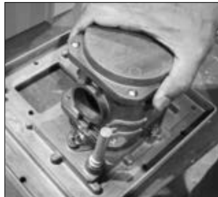
Figure 16.10 Example - Proper alignment of measurement cartridge
