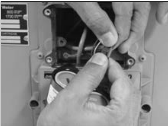
Figure 9.8 Example - Remove battery
