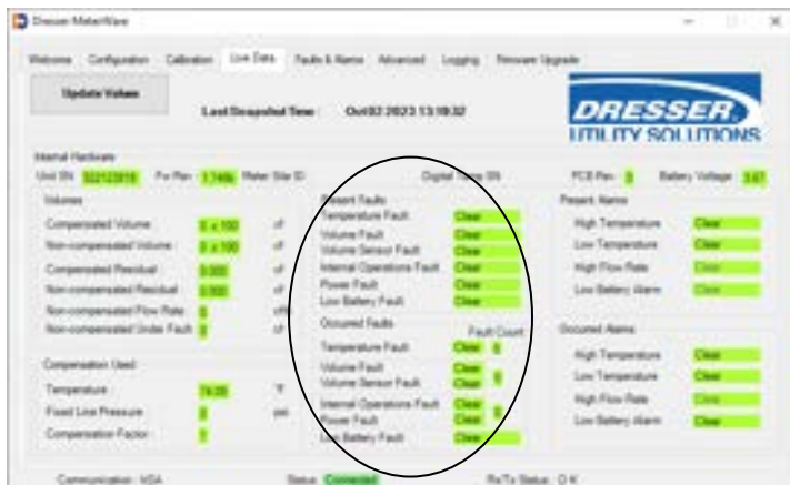
Figure 8.2 Example - Live Data Screen showing Faults in Dresser MeterWare Software
