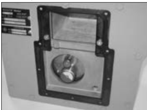
Figure 9.13 Example - Place gasket onto meter
