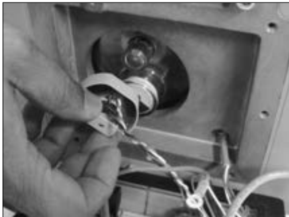
Figure 9.12 Example - Remove Wiegand assembly.
