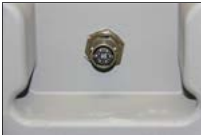
Figure 7.15 Example - Pulse output cable on backside of meter
