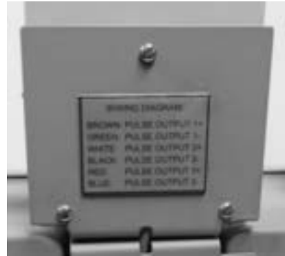
Figure 7.32 Example - Cover Plate with Wiring Guide
