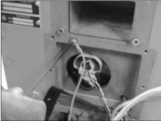
Figure 9.11 Example - Remove green ground wire
