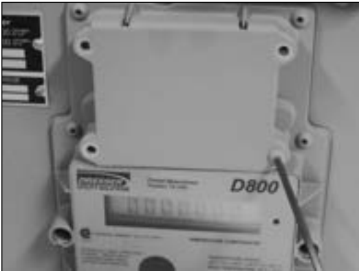
Figure 9.7 Example - Remove 4 screws on battery compartment
