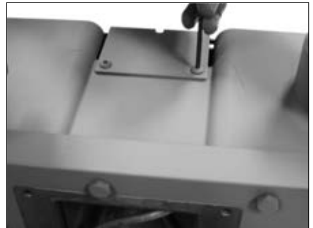
Figure 9.10 Example - Remove AMR plate
