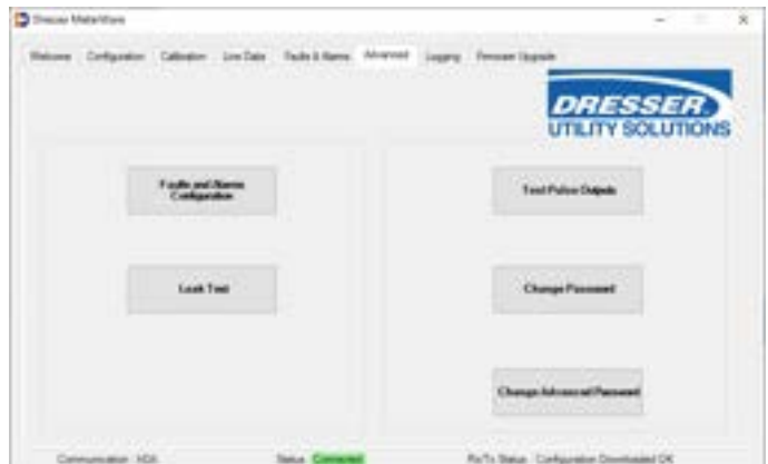
Figure 7.11 Example - “Advanced” screen of the Dresser MeterWare software
