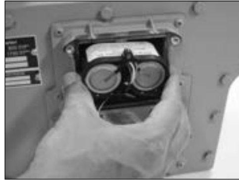
Figure 9.21 Example - Place battery inside compartment
