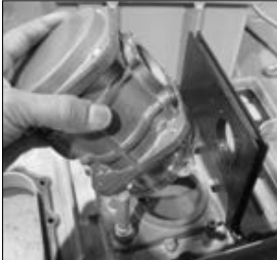
Figure 16.7 Example - Remove Cartridge
