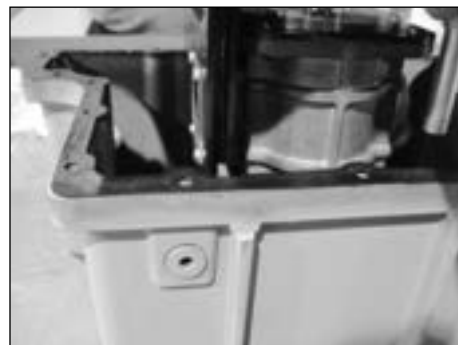
Figure 16.16 Example - Aligning gasket slots with ribs
