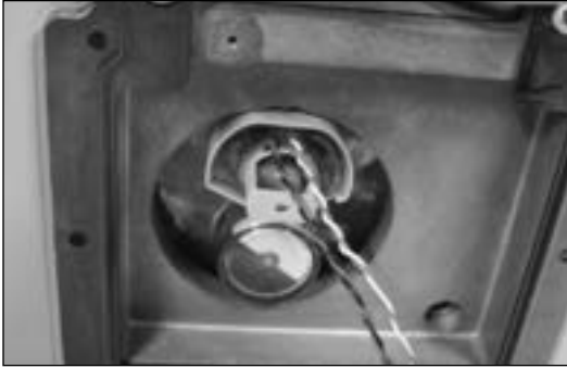
Figure 9.17 Example - Place Weigand into compartment
