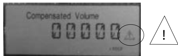
Figure 7.31 Example - Fault/Alarm symbol as displayed on LCD Screen
