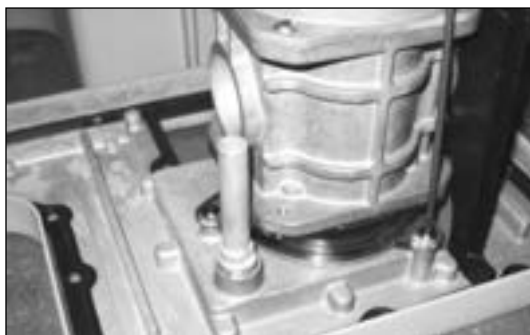
Figure 16.5 Example - Remove 3 (#10-24) screws
