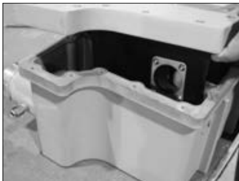
Figure 16.3 Example - Pull front enclosure off
