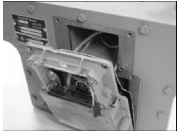
Figure 9.9 Example - Pull index away from the meter
