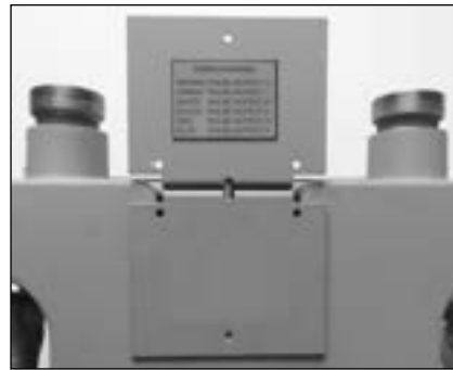
Figure 7.17 Example - Properly positioned mounting bracket
