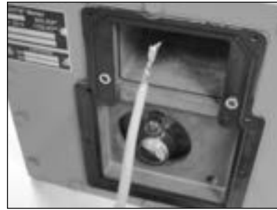
Figure 9.14 Example - Pulse output cable
