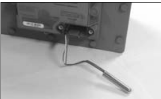
Figure 9.19 Example - Temperature probe extended through the front of the instrument cover
