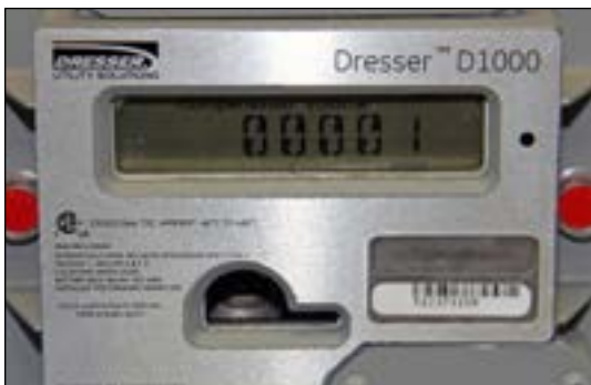
Figure 6.1 Example - Label on D1000 meter
