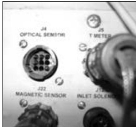
Figure 10.12 Example - Optical sensor port (J4) with and without the connector.
