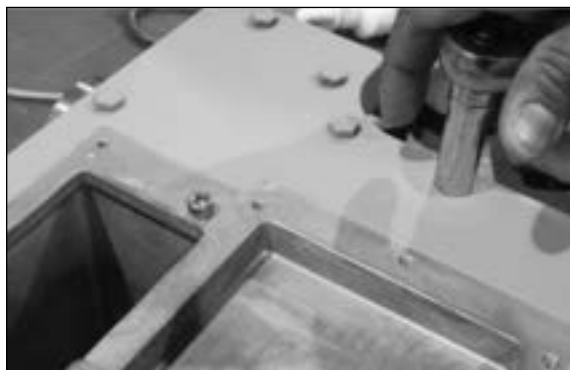
Figure 16.1 Example - Remove the 16 bolts
