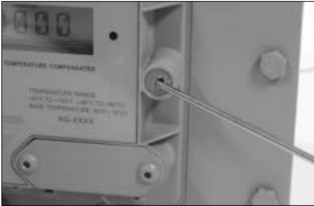
Figure 9.6 Example - Remove rock seals.
