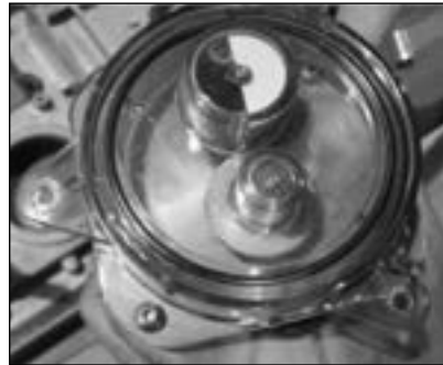
Figure 16.9 Example - Place O-ring on amber cartridge cover
