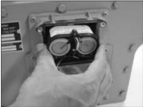
Figure 9.28 Example - Remove battery pack
