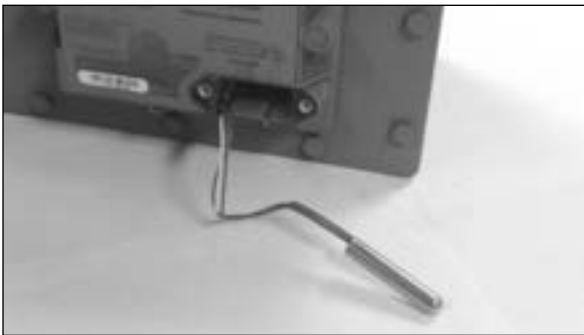
Figure 9.2 Example - Temperature probe removed from compartment
