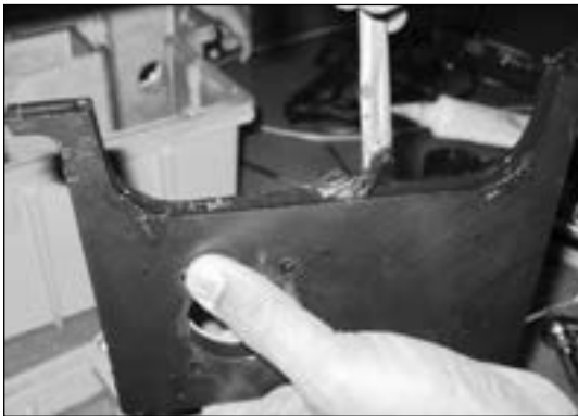
Figure 16.12 Example - Apply grease to gasket
