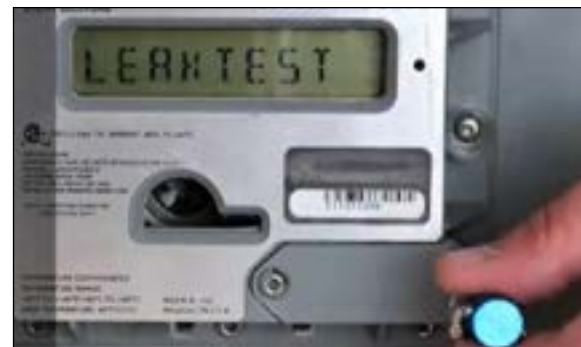
Figure 7.7 Example - Scroll to LEAKTEST screen
