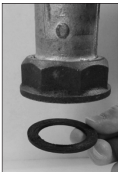
Figure 7.1 Example - Proper installation of washer into swivel
