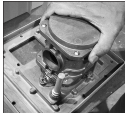
Figure 16.10 Example - Proper alignment of measurement cartridge
