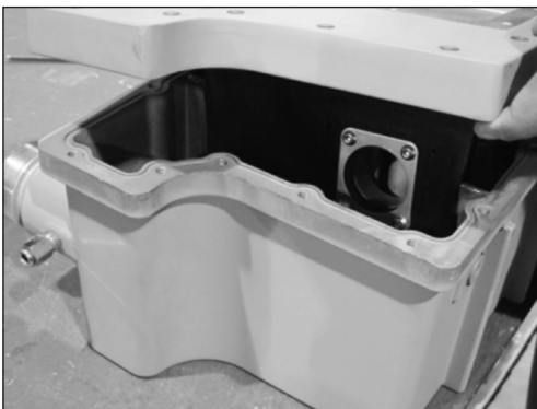
Figure 16.3 Example - Pull front enclosure off
