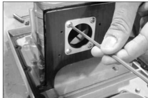
Figure 16.6 Example - Remove 4 (#10-24) screws on main gasket
