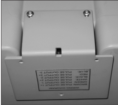
Figure 7.14 Example - AMR mounting brackets as shipped from factory
