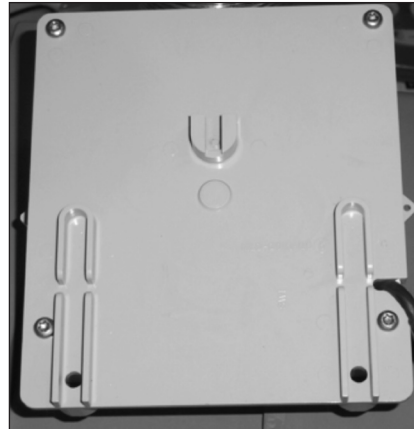
Figure 7.23 Example - Attach ERT to backplate with Torx screws
