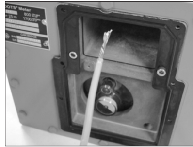
Figure 9.14 Example - Pulse output cable
