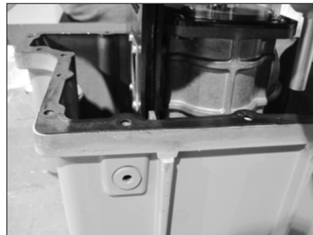
Figure 16.16 Example - Aligning gasket slots with ribs
