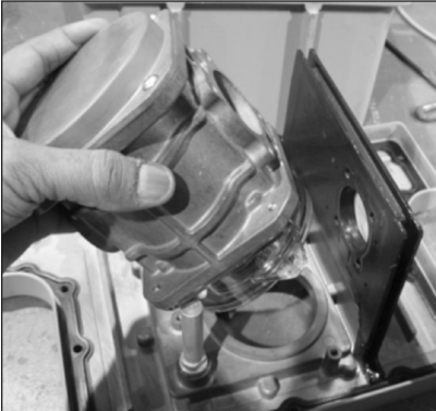
Figure 16.7 Example - Remove Cartridge
