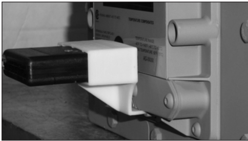
Figure 10.15 Example - IrDA adapter placed into slot
