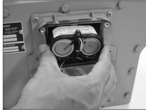
Figure 9.21 Example - Place battery inside compartment
