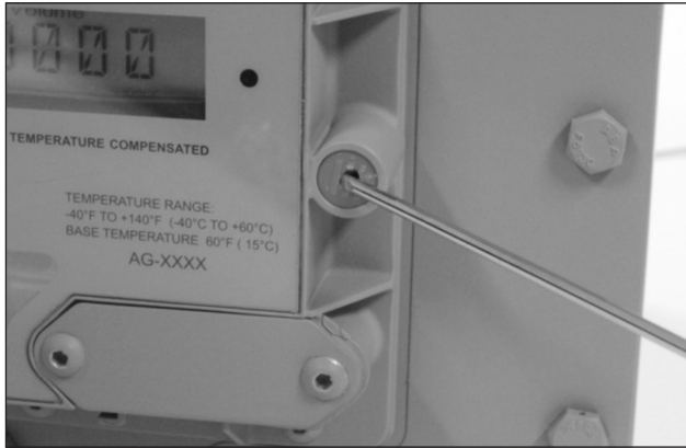
Figure 9.6 Example - Remove rock seals.
