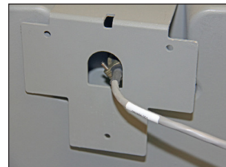
Figure 7.18 Example - Pull cable through the center hole
