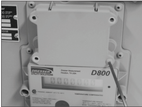
Figure 9.27 Example - Remove 4 screws on battery cover
