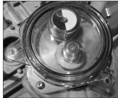
Figure 16.9 Example - Place O-ring on amber cartridge cover
