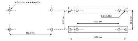
Figure 1 - Fixing dimensions
