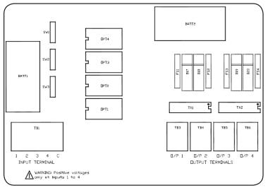
Figure 2 – Electrical Connectivity
