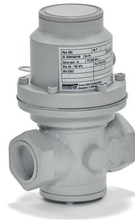
The SRV 803 relief valve is installed downstream of pressure regulators to relieve limited volumes of gas. Used where venting to the atmosphere is acceptable, it provides a cost-effective solution to prevent safety shut-off valves from triggering in case of creep leaks from regulators. This valve is ideal for medium pressure settings and offers a wide setting range and robust performance.
