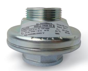
The SERus and SERus E residential regulators are based on a spring-loaded measuring unit. This type of regulator is used for direct pressure regulation at the inlet of residential and industrial gas meters.
