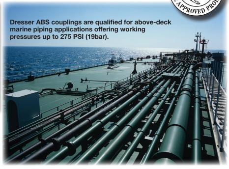
Dresser couplings are widely used for marine piping systems for their ability to absorb vibration, expansion and contraction while providing leakproof dependability.
