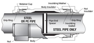
NOTE: These Style 90's are compliant to Category 1 requirements for plastic pipe joints. However, as shown in above illustration only steel pipe can be used on the Insulating End
