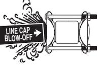
Style 31 Line Caps **MUST NOT** be used under pressure without anchorage or blocking sufficient to withstand the entire longitudinal thrust due to internal pressure. Failure to do so could allow line cap to blow off the line, causing serious injury or death. Also, escaping line content could cause property damage, serious injury or death.
