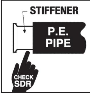
NOTE: On all polyethylene pipe ends, the recommended Dresser insert stiffener, or an insert stiffener the user has qualified to meet CFR Title 49, DOT 192.283(b), must be installed.
