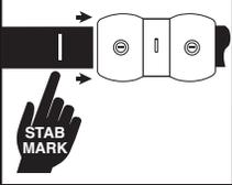
You **MUST** mark and stab the pipe into the coupling to the proper stab depth. Failure to do so could result in escaping gas that could ignite and cause property damage, serious injury or death.
