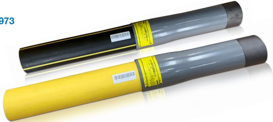
Dresser introduces the Style 721 Transition Fitting for quick, reliable Steel to PE transition connections for gas distribution mains. They are engineered for full compliance with the attendant gas distribution industry standard ASTM F1973. The Style 721 steel bodies are coated with Dresser ALCLAD™ fusion bonded epoxy with 2" layback for field welding. The weld end comes factory-beveled.
