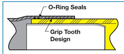
The gripping design is based on the features utilized successfully for decades in the Dresser Style 711 Universal mechanical coupling product line. The gripping tooth profile has been proven by extensive field use and most recently in qualification testing of these mechanical coupling products to the requirements of ASTM F1948, which closely align to those in F1973.
