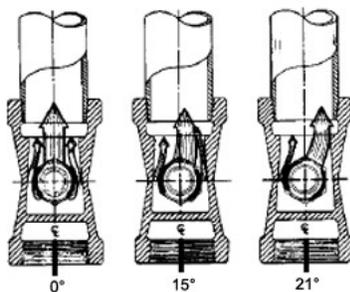
8. Verify the orifice retention beads seat against the orifice (see the following Loading Ring Position table).
