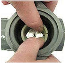
5. Remove the orifice using a 1 7/16-inch thin-wall socket wrench.
