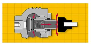
A. Standard regulator and upstream monitor orifice.
