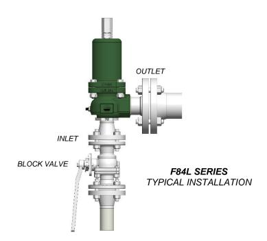
The F84L Series valves are balanced against superimposed backpressure, so that the set pressure will not change with backpressure.
