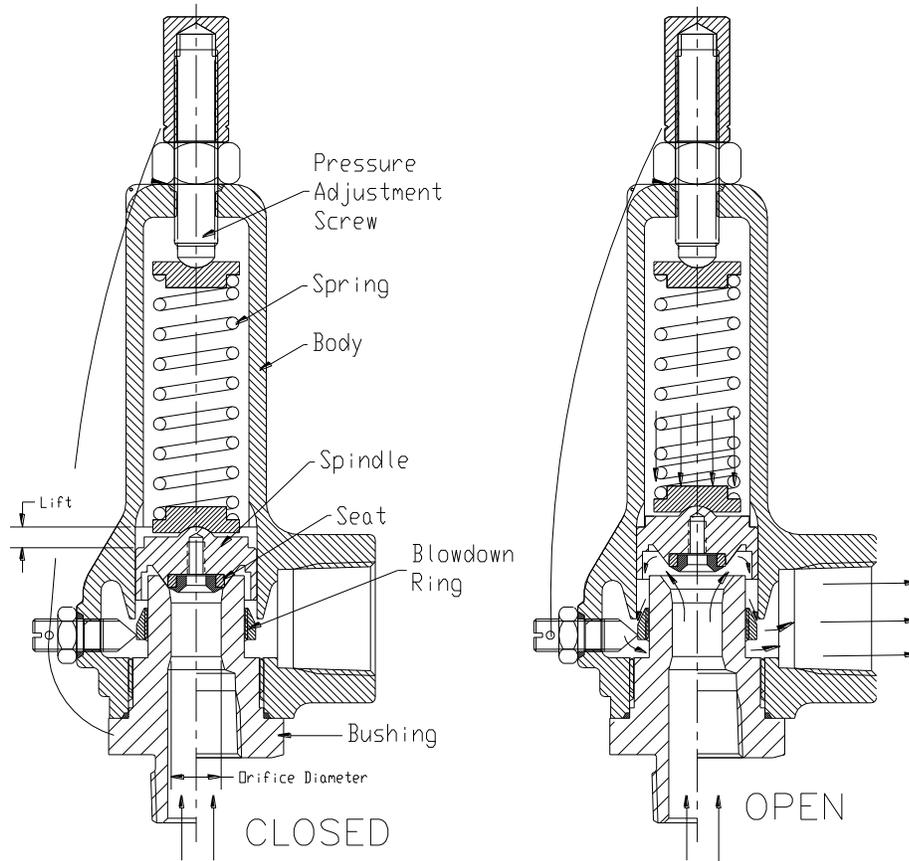
The FLOW SAFE F80 Series safety relief valve is a direct-acting spring-loaded relief valve, suitable for gas service. The Type F84 is plastic-seated and the F85 is elastomer-seated.
