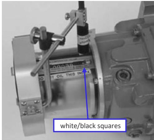
Figure 16: Optical Scanner relative positioning and alignment, Series B3 accessory unit
