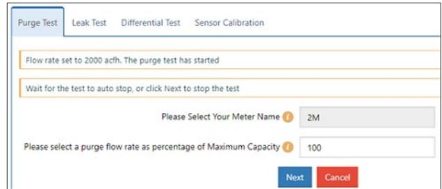
Figure 93: Purge test running
