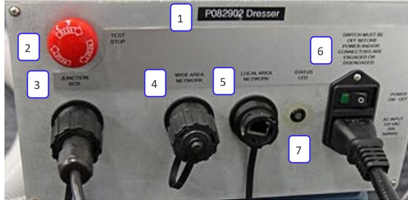
Figure 3: Controller Connections and Test Stop button
