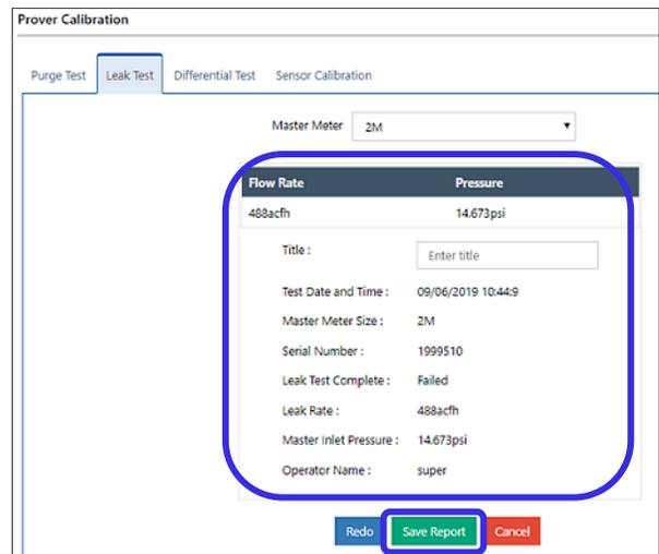
**Figure 103: Leak test complete**
