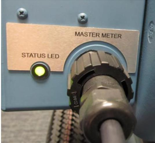
**Figure 6: Verify Master Meter communication cables connected**
