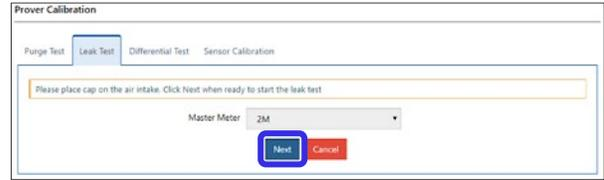
**Figure 101: Cap the air intake and start leak test**
