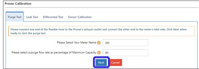
Figure 92: Check connections, and start purge test
