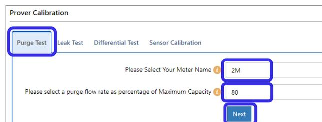
Figure 91: Purge test settings tab
