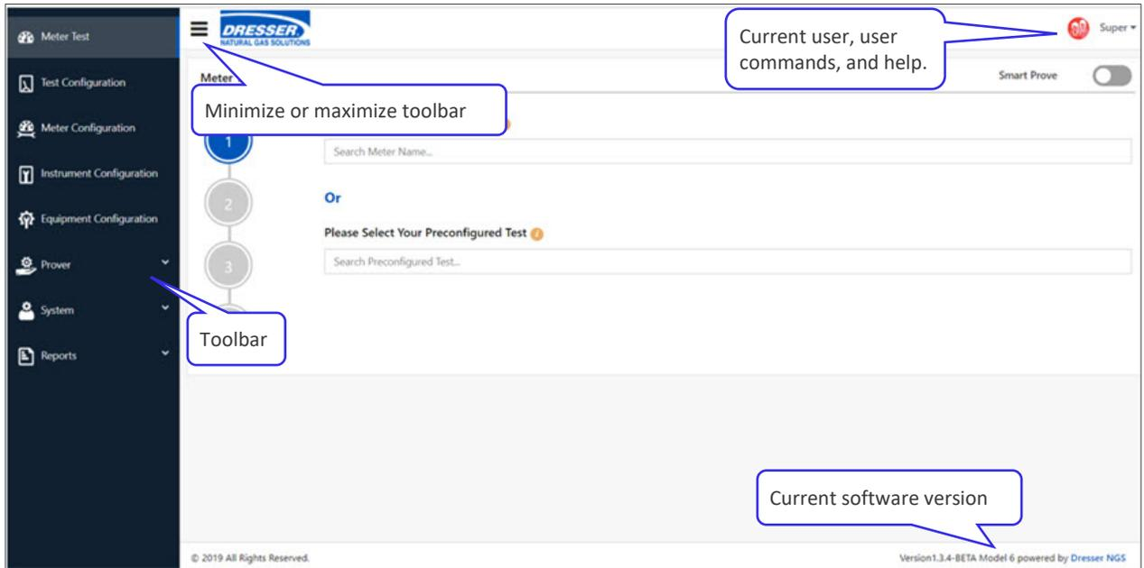
**Figure 32: Model 6 Prover software screen features**
