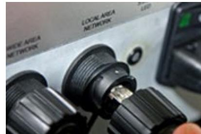
**Figure 22: Connect with an Ethernet cable**
