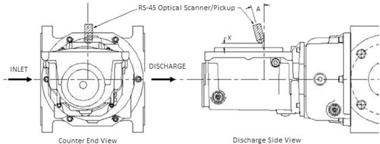
**Figure 20: Optical Scanner relative positioning and alignment, Series B2 (TQM) accessory unit**
