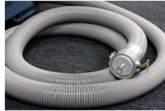
Figure 96: Cap the air inlet of the Field Meter
