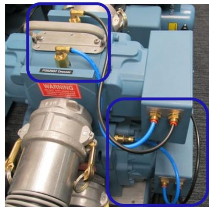
**Figure 9: Master Meter pressure lines connected**
