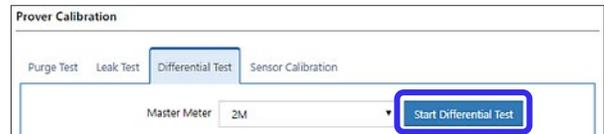
Figure 107: Click Start Differential Test to begin test
