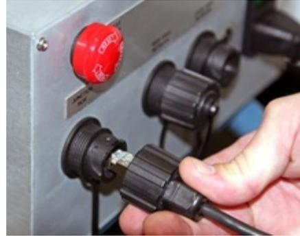
**Figure 11: Connect Junction Box Ethernet cable to the Controller**
