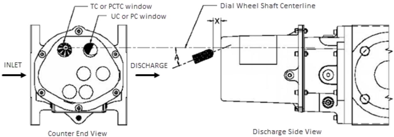
Figure 19: Optical Scanner relative positioning and alignment, Series A1 (LMMA) accessory unit
