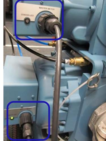
**Figure 7: Master Meter communication cables connected**
