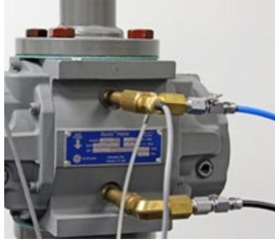
Figure 12: Field Meter with ID Pulser attached
