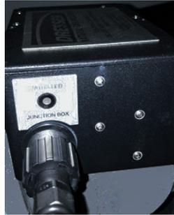
**Figure 10: Connect Ethernet cable from the Field Meter Junction Box**
