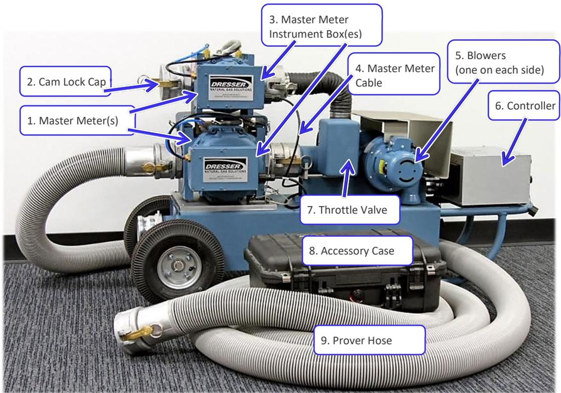
Figure 1: 10M or 2M/10M Prover parts identification
