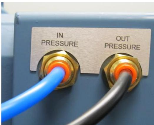
**Figure 8: Master Meter blue inlet and black outlet pressure lines connected**
