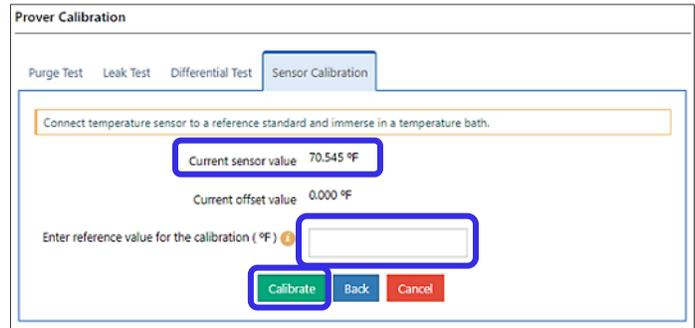
Figure 118: Sensor Calibration Connect sensor screen
