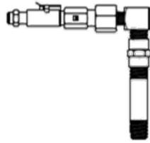
**Figure 128: Pressure Adapter
