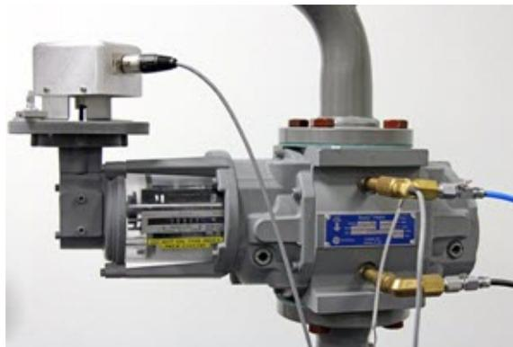
Figure 14: Instrument Drive Pulser test setup
