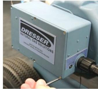
Figure 114: Remove cover plate on Master Meter
