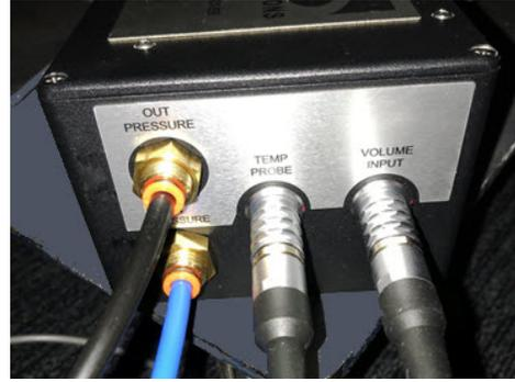
Figure 13: Attach blue inlet and black outlet pressure lines
