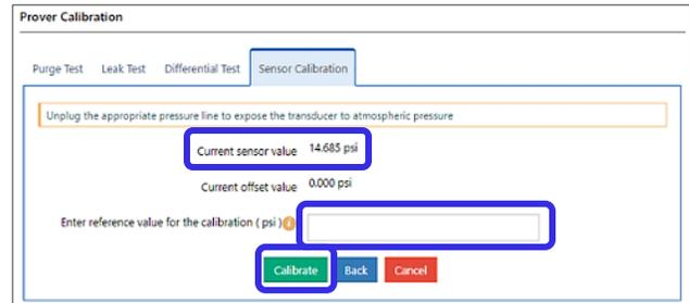
Figure 121: Pressure Sensor Calibration tab
