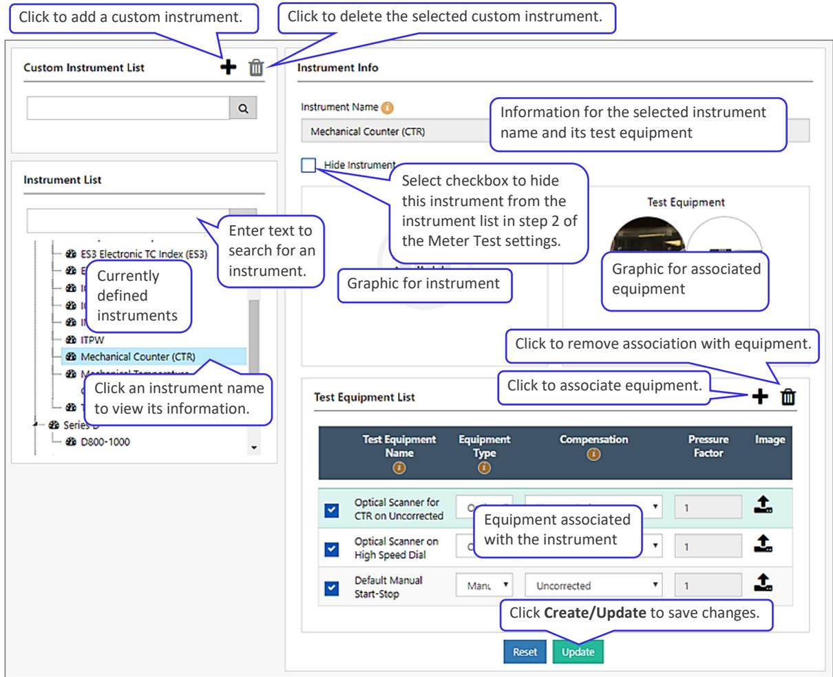
Figure 64: Instrument Configuration screen
