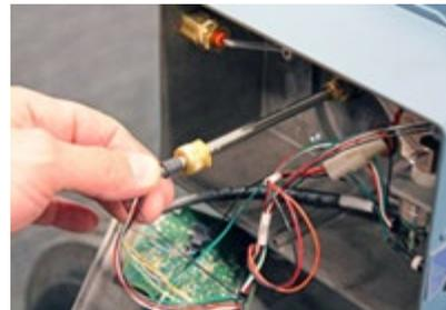
Figure 115: Remove Master Meter temperature probe
