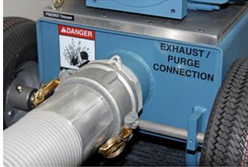
Figure 89: Prover exhaust purge outlet
