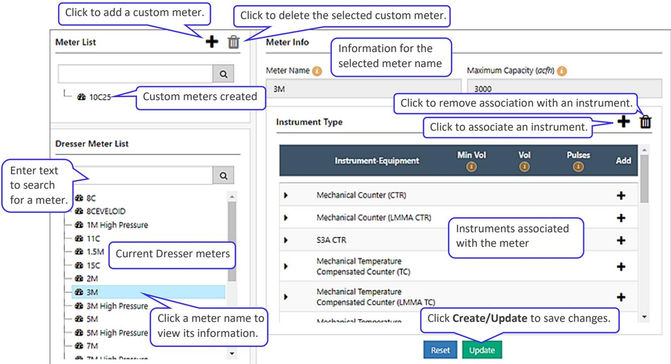
Figure 73: Meter Configuration screen
