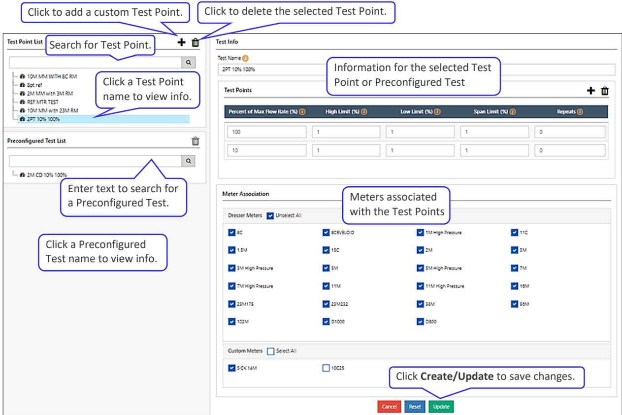
Figure 82: Test Configuration screen
