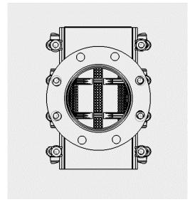
Opposing seal beads in upper and lower gaskets provide secure 360 degree sealing against full break pipe. Shell, Aperture Seal and Seal Bead Geometry are Patent Pending.
