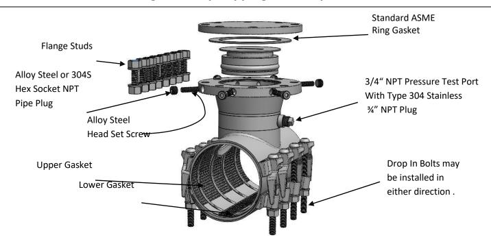
Flange Studs: Sized to match ASME B16.5 flange bolt specifications/requirements.
