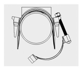
Hinge geometry provides extra opening/spreading range on 4" thru 8" diameter sizes.
