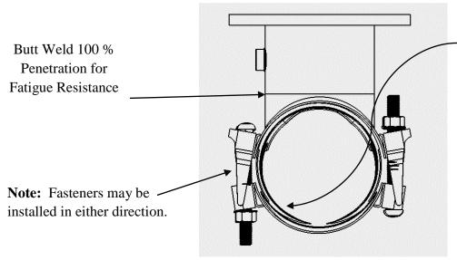
Special patent pending contoured seal beads and molded aperture seal provide for extended range capabilities. Patent applied for.
