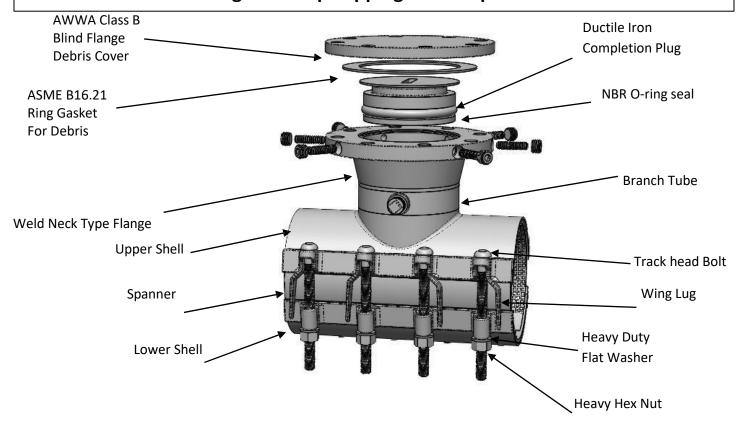
Flange: Epoxy Coated Carbon Steel or 18-8 Type 304 Stainless Steel,
