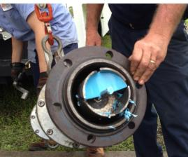
Triple Tap Tapping Sleeves and Line Stop fittings are tested to meet ANSI/AWWA C223-07 and MSS SP-124-2012. In addition, consideration is made to the various pipe materials used in the pipeline industry including: steel, cast iron, ductile iron, PVC, High Density Polyethylene, Asbestos Cement and Copper Pipe.
