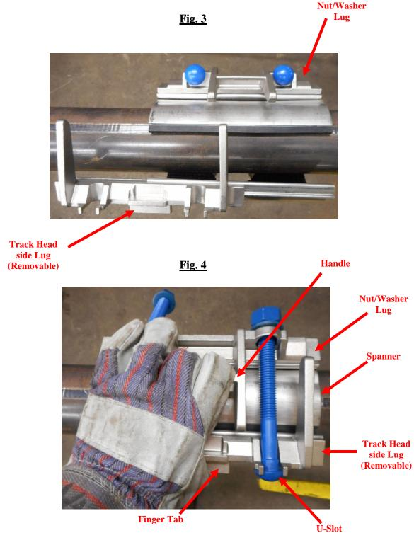
**Step 5.** Insert the remaining bolt into the corresponding U-slot. Ensure nut sides of the bolts are secured through the closed holes on Nut/Washer Side Lug. The track head should nest securely behind the two bolt head retaining tips on the track head U-slot. (See Fig. 5) Once the bolts are secured in the bolt slots, but not yet tightened, rotate the saddle to the desired orientation.
