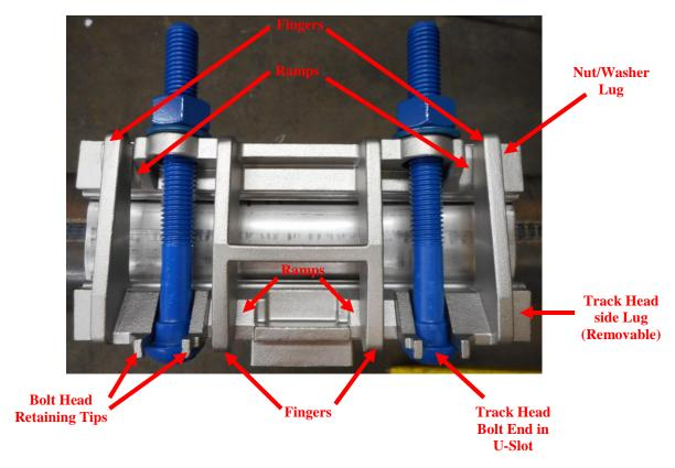
**Step 5.** Tighten the nuts evenly (maintaining an even gap) to correct torque per requirements (Next Page). As the Fitting is tightened, verify that the lug fingers travel along their corresponding/mating ramps. (See Fig. 5)
