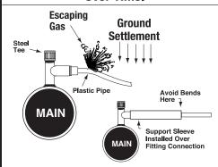
To limit shear and bending stresses at the mechanical fitting connections, the use of a support sleeve is recommended to provide support from the effects of ground settlement. Bends at support sleeve exit should also be avoided. Failure to properly compact the soil and use a suitable support sleeve could result in escaping gas that could ignite and cause property damage, serious injury or death.
